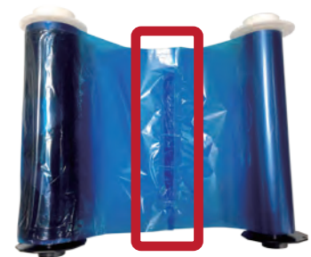
Tape the ribbon back together , and place ribbon back onto cartridge. Make sure to scroll the ribbon back onto the cartridge as tight as possible, till the broken part of the ribbon cannot be seen.
