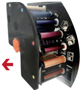
Step1. Turn off printer, open and pull out ribbon door. Make sure to separate ribbon cartridge from the printer, if ribbon is jammed into the printer, please cut it loose. *
